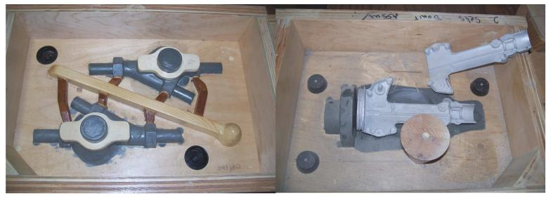
These two matchplates are part of Bud Statton's Vietnam-era flamethrower reproduction project. The one on the left is the valve that controls the fuel distribution and the other is part of the trigger assembly. Below are some castings that came out looking nice. Below to the right is a core box for molding the threads above.
