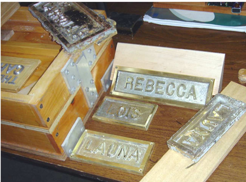
To the left are some brass plaques created by Bud Statton for family and friends. Much effort went into adapting the gating and runners to the flow characteristics of the material. The results show it was quite worth it. The grey patterns on the right are the forward housing for his flamethrower reproduction project.
