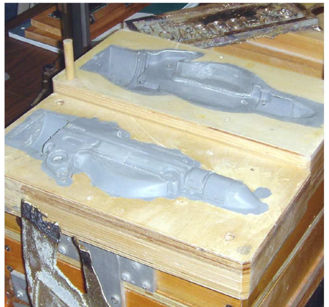
To the left are some brass plaques created by Bud Statton for family and friends. Much effort went into adapting the gating and runners to the flow characteristics of the material. The results show it was quite worth it. The grey patterns on the right are the forward housing for his flamethrower reproduction project.
