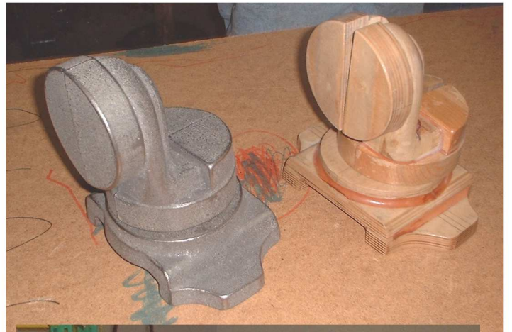
At right, a set of patterns for a Cincinnati Milacron grinder bracket. They were built by John and Trudy Benjamin. Poured at Silverton foundry in cast iron, they were tumbled to clean off any scale and are ready for machining.
