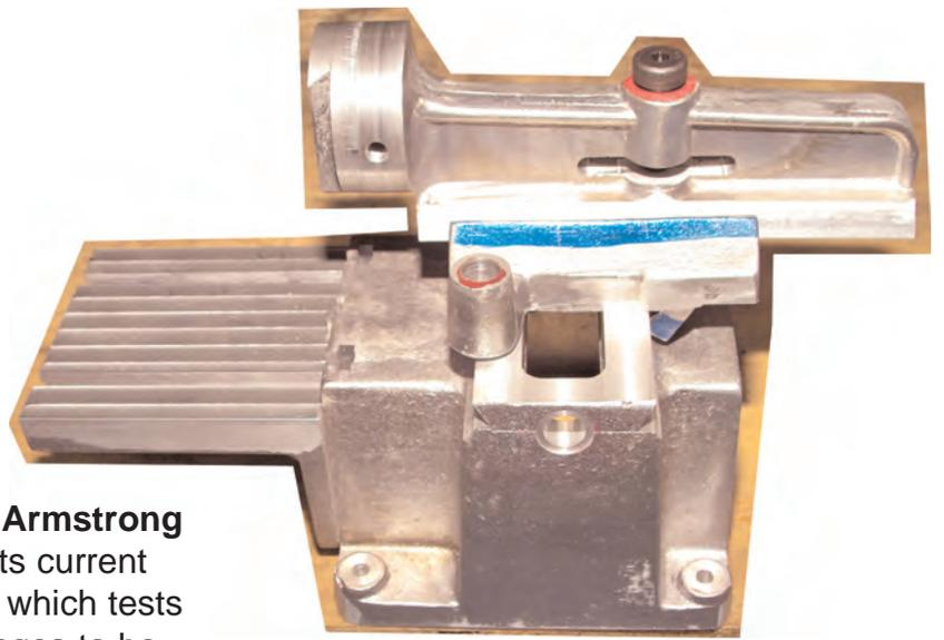
**Tom Hammond** brought the partially finished **Armstrong** hand shaper shown above and right to show its current status . This aluminum version is a prototype which tests how well the parts fit together and allows changes to be made before the iron versions are cast. This low weight version will also be used by **Gary Martin** to take to model engineering shows. It is expected that some casting kits will be available for sale. The saga continues.
