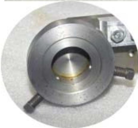
moved manually in a circle cutting a spherical shape. Tom didn't say if he used this to cut the ball handles in a quorn.
