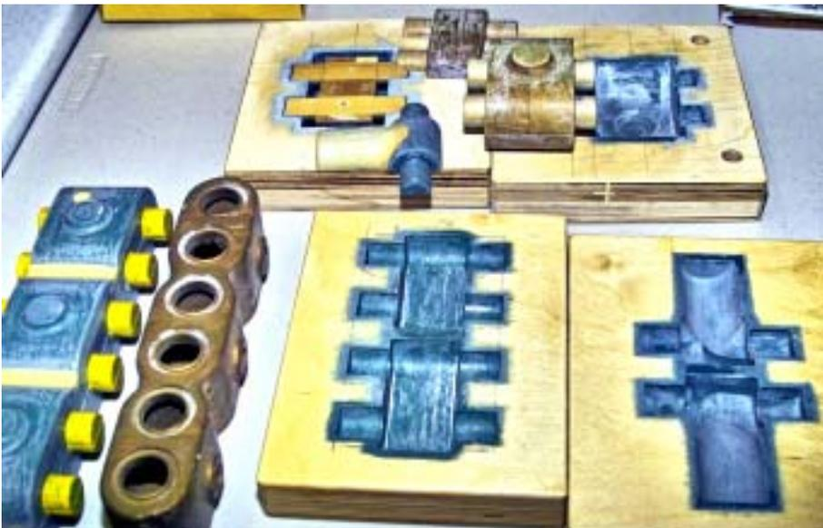
**Gary Martin** brought the molds (at left) for the 1910 Holt caterpillar tractor parts he has been contracted to make.
