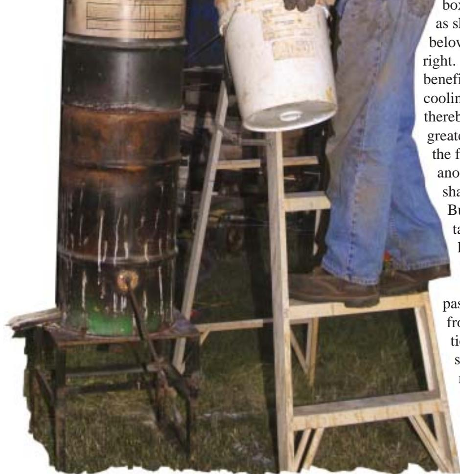
For example, he showed us the economies of using a single hole for both air feed and the pouring spout (as shown at right) Not a single member was smart enough to figure this out by himself.
