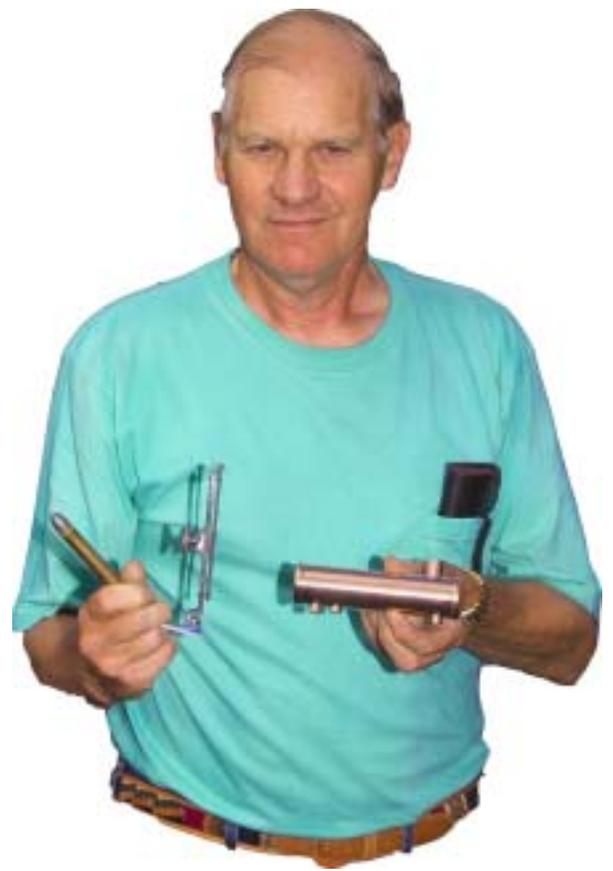
**Tom Hammond** brought his latest ebay steal (above). Its a machinist microscope of extraordinary construction. The table has T slots, micrometer positioners and spring loaded slides to remove all vestiges of backlash.
